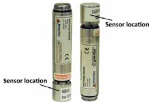
Figure 2. A Pair of Data Loggers Measuring High and Low Locations Within the Sterilization Bag
